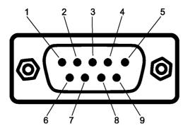
Figure 4. The DSUB connector on a DRVcan.
